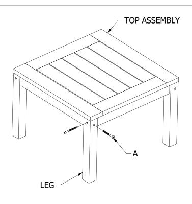
1) Attach leg to table top using (2) A bolts. Drilling a 3/16" pilot hole first will assist in driving the bolts.
